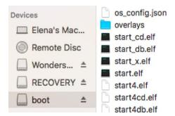
To enable SSH on raspberry Pi just place a file named "ssh" on the card.
