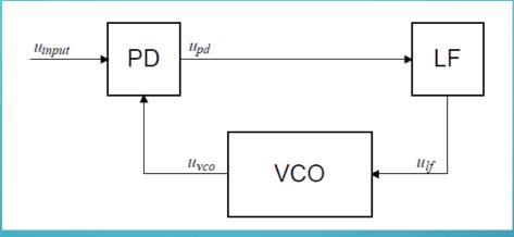
As a phase detector a simple multiplier can be used, which multiplies the input with the output of the voltage controlled oscillator and the result will be the sum of a DC with a time varying component.
