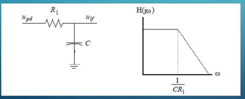
The transfer function for the filter will be given by:
