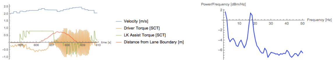
Figure 4.7: A plot of how the go-kart is led back to the lane by the lane keeping assist. As a side effect, oscillation occurred. On the right, the corresponding power spectral density diagram is displayed.
