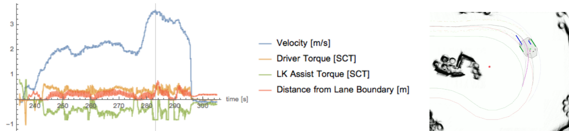
Figure 4.4: Appearance of the biggest error among the evaluated data, while the maximum applied driver torque is smaller than 0.8[\text{SCT}]
