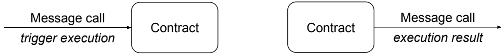
(a) Message call to a contract account which trigger the execution of code.
